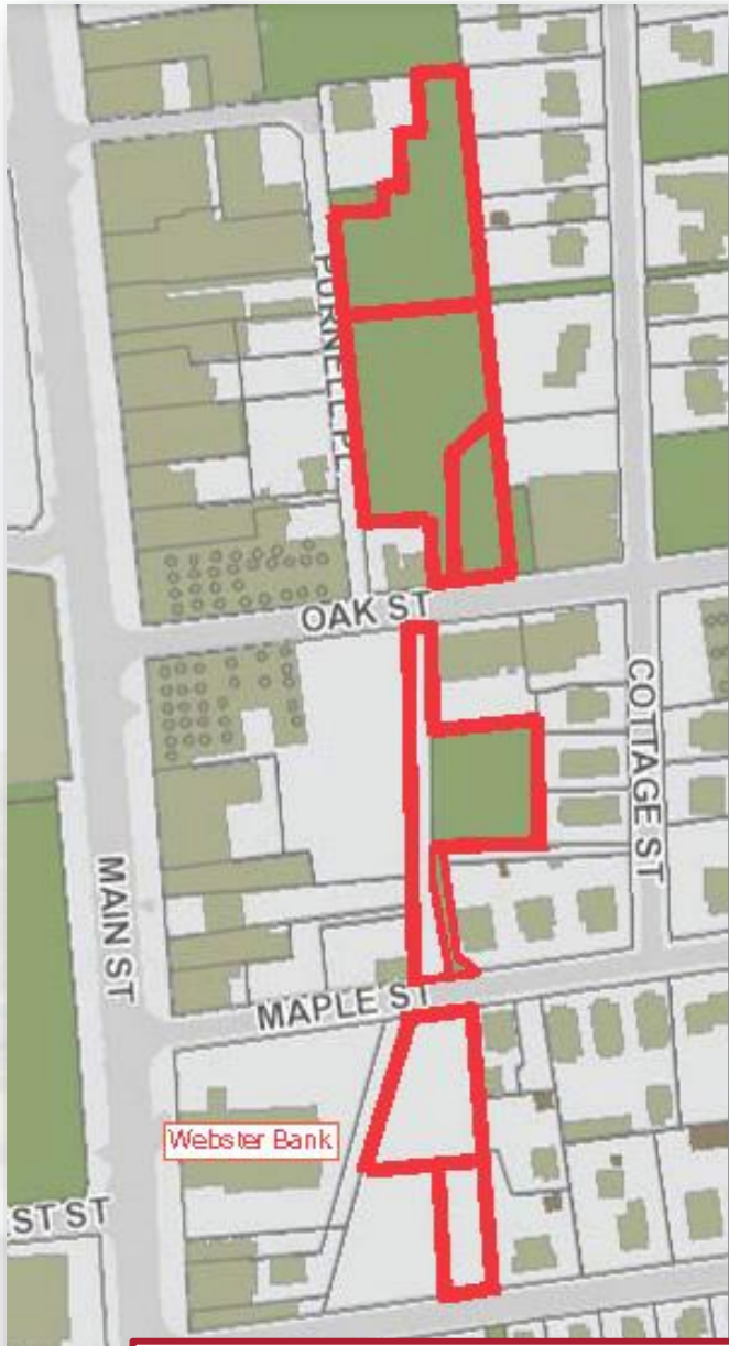
Geothermal Heat pumps Test fit wellfield on project parcel and adjacent Town-owned sites
