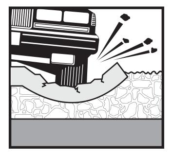
When vehicles drive over this cavity, the pavement surface cracks and falls into the hollow space, leading to the birth of another pothole.
