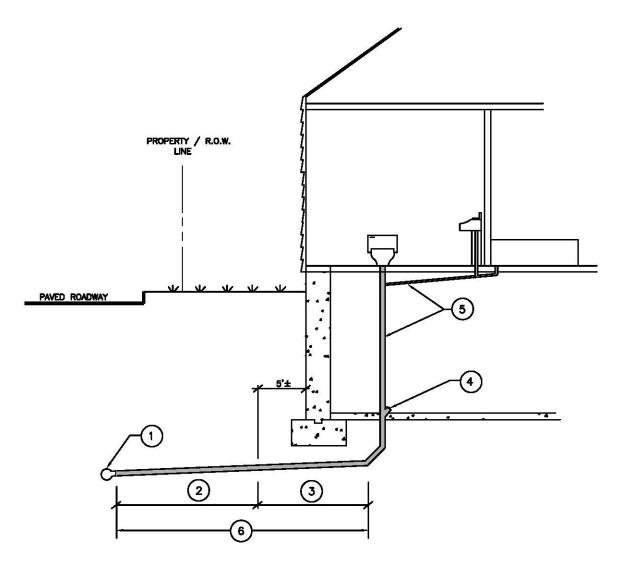
NOTE: THE SHADED PORTIONS OF THE SYSTEM CONSTITUTE THE SANITARY SEWER LATERAL AND THE DOMESTIC WASTEWATER SYSTEM AND ARE OWNED, OPERATED, MAINTAINED, REPAIRED, AND REPLACED BY THE OWNER
