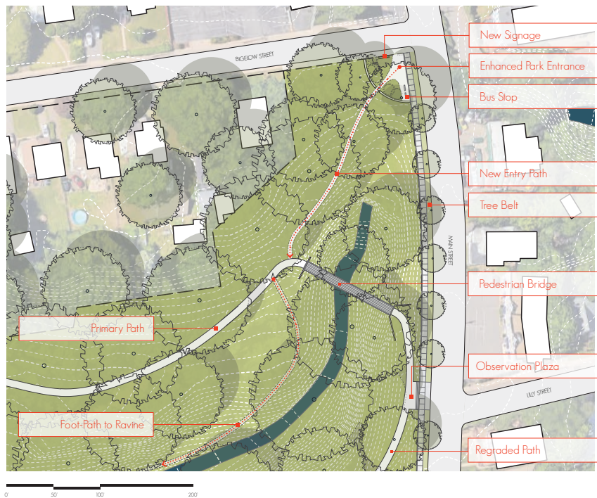
Figure 29: A pedestrian bridge would serve as both an observation deck and as part of the park trail network, connecting the major north and south trails.
